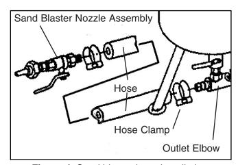
**Figure 4.** Sand blaster hose installation.
